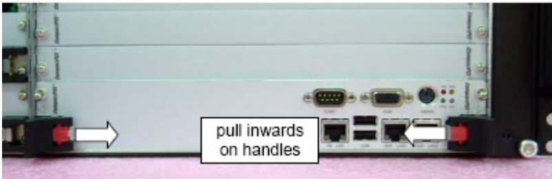
Figure 2-2: Latching the cPCI module handles securely.
