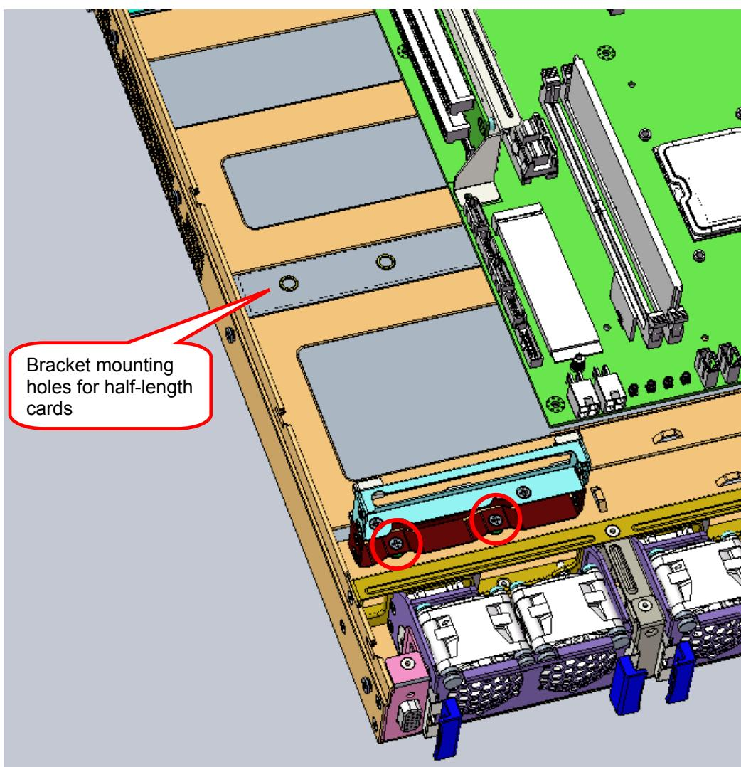
5. First install the lower PCIe expansion card. Align the tab on the bracket with the opening on the rear I/O panel (A), and insert the PCIe connector into the slot on the riser card (B). Make sure the connector is fully inserted into the PCIe slot.
