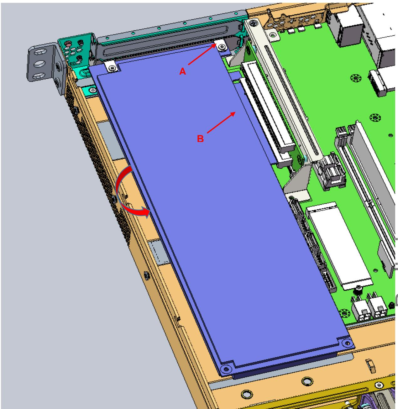
6. Then install the upper PCIe expansion card, if required
