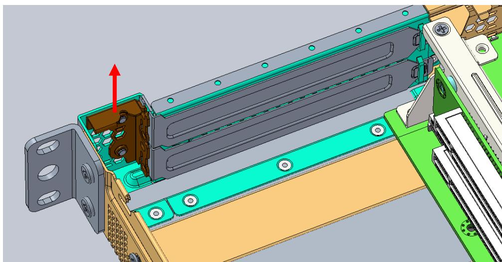
3. Remove the PCIe bracket blanking plates.
