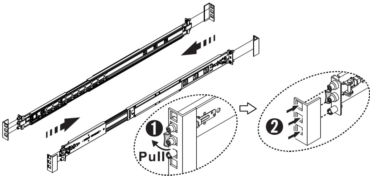
**Note:** Front and rear bracket detachment procedures are the same. The left and right sides of the rail are symmetrical. Repeat the steps for the other side.
