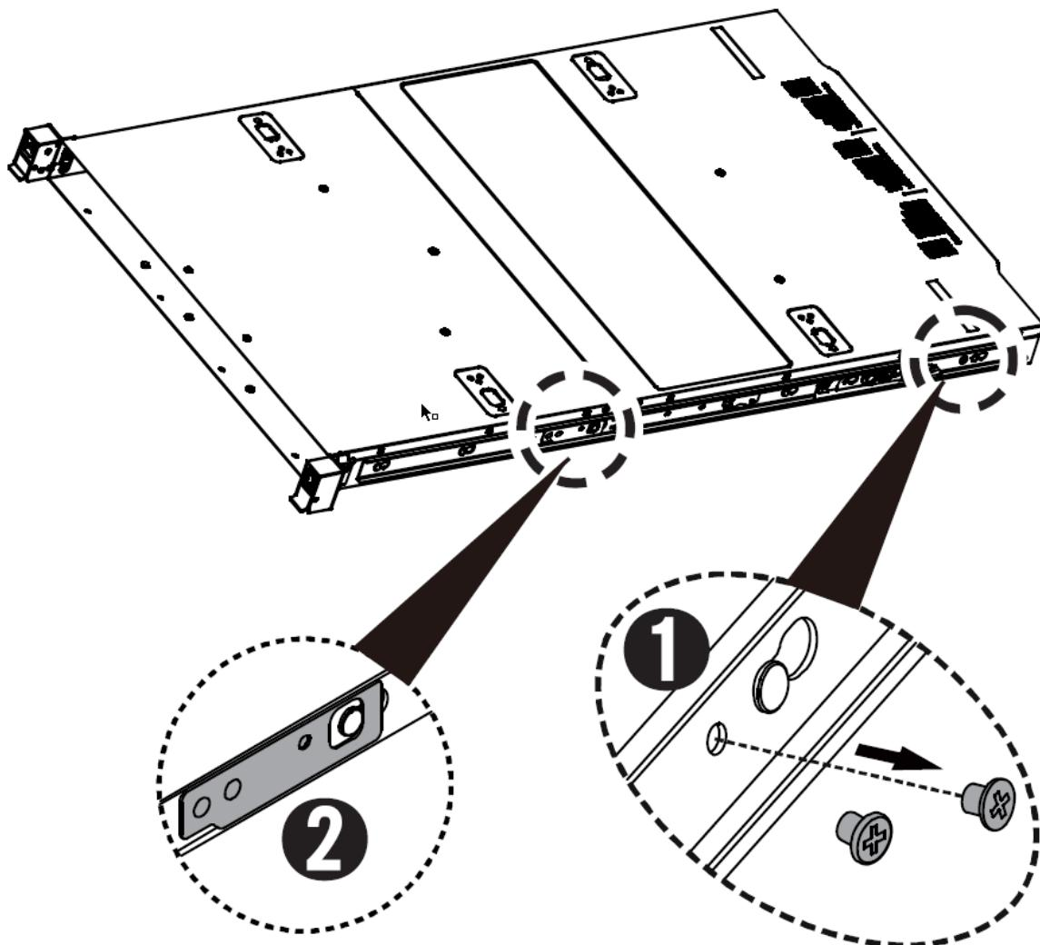
Detach the outer rail/bracket assembly from the rack.
