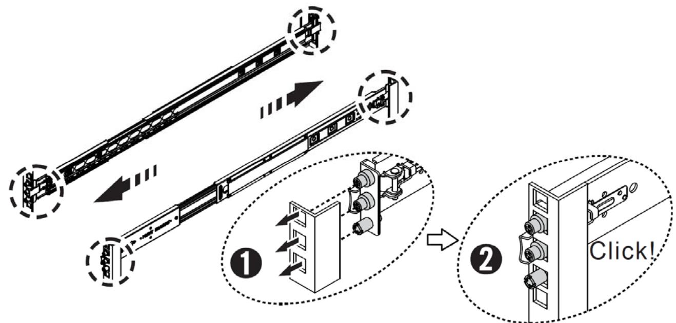
**Note:** Front and rear bracket installation procedures are the same. The left and right sides of the rail are symmetrical. Repeat the installation steps for the other side.
