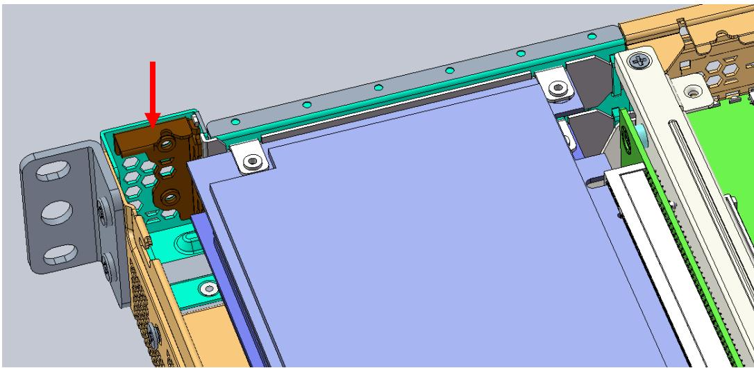
9. Secure the bracket with two screws as shown.
