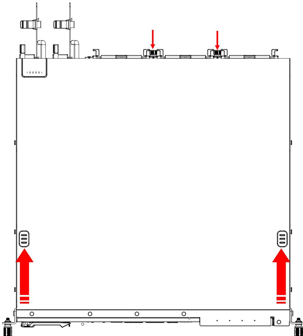
To reinstall the cover, slide it towards the front of the chassis, then tighten the screws loosened in Step 1.
