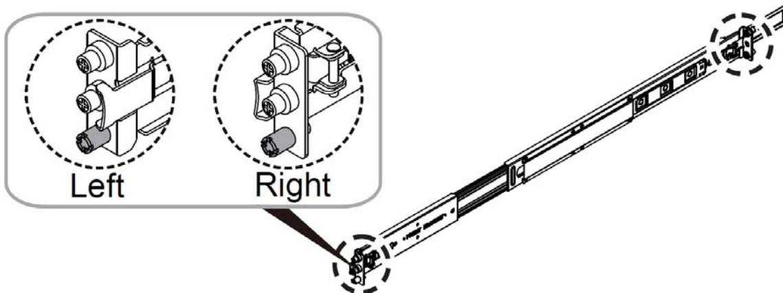
To switch from round hole to square hole, remove the "A" type screws (pre-installed) and switch to "B" type screws.
