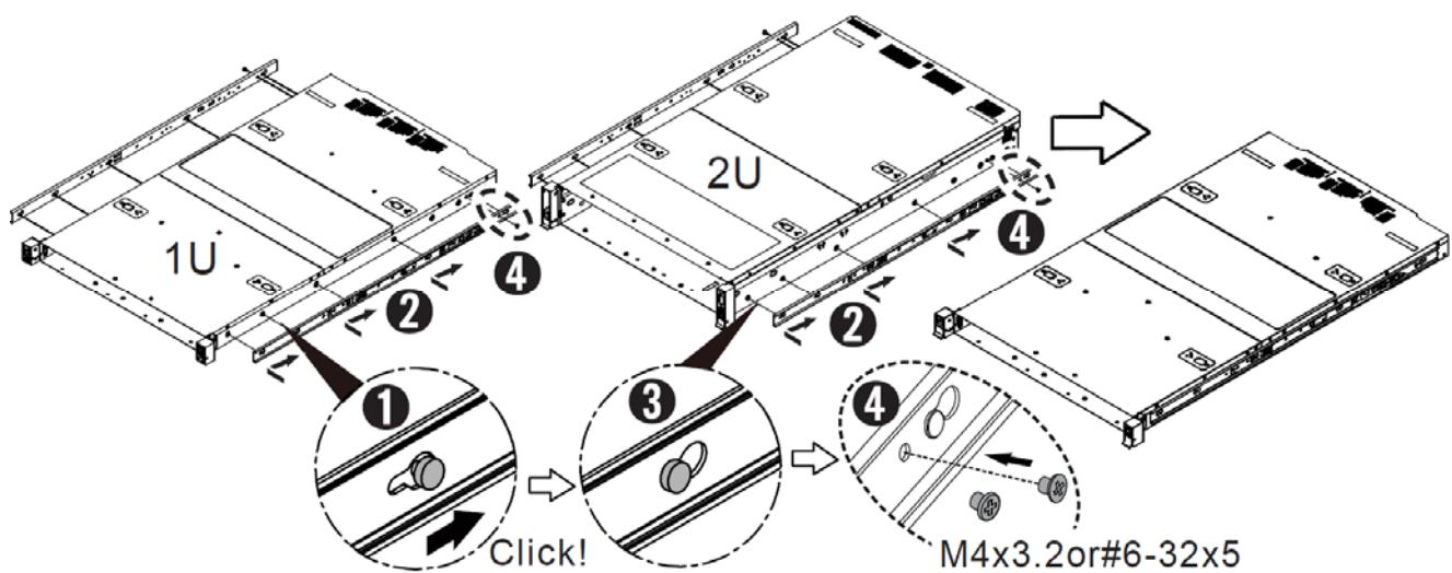
3. Attach the outer rail/bracket assembly to the rack.
