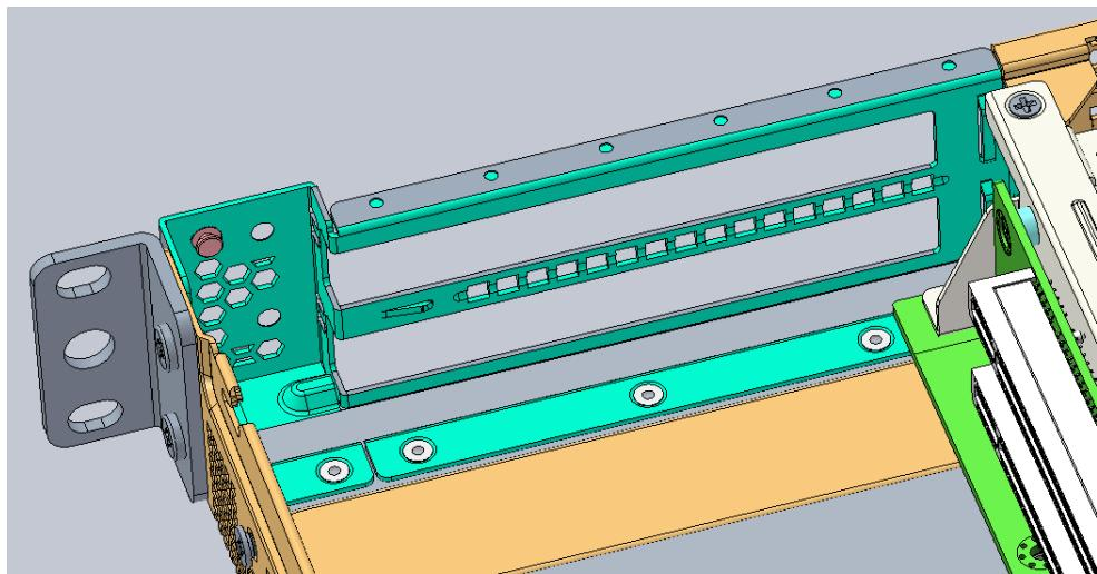
4. Loosen the two screws to remove the internal PCIe bracket used to secure the PCIe cards inside the chassis. The diagram shows the position of the bracket for full-length cards.
