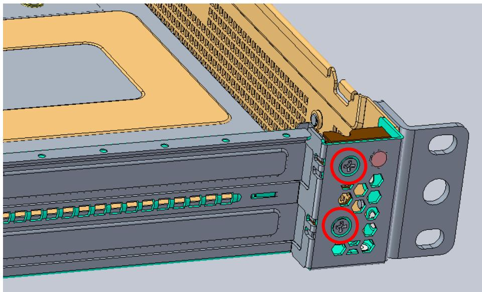
2. Remove the bracket securing the PCIe bracket blanking plates.
