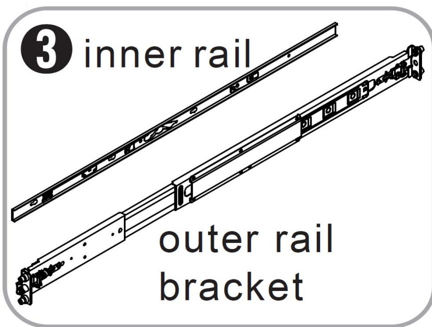
2. Install the inner rail onto the chassis.
