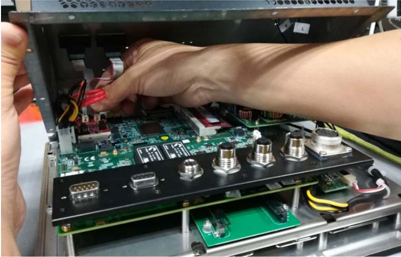
5. Reconnect the cable connecting the speakers to the main board, reinstall the rear cover onto the device, and secure the cover by replacing the screws. Replace the USB slot cover.
