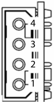
**Figure 1-11: 4 Pin 12V Power Connector**
