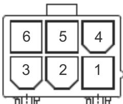
Figure 1-12: 6 Pin 12V Power Connector
