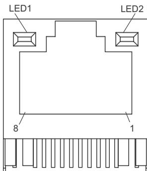
**Figure 1-9: RJ-45 Ethernet Connector**
