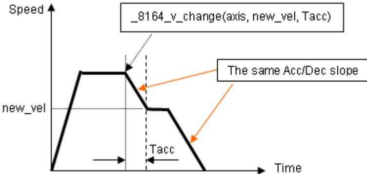
The change speed on the fly function is only applicable for single axis motion. Both velocity mode motion and position mode motion are acceptable. The graph above shows the basic operating theory.
