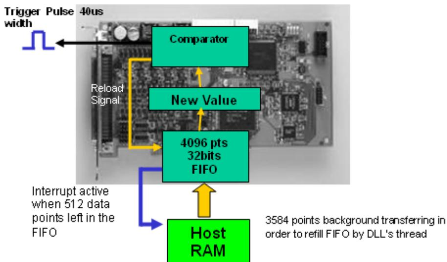
The **Value** block in this figure is the position where the comparison occurs, and where the data can be checked by using `_8164_check_compare_data()`.
