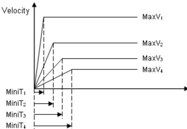
How do users decide an optimum value for “OverVelocity” in the `_8164_fix_speed_range()` function? The `_8164_verify_speed()` function is provided to calculate such value. The inputs to this function are the start velocity, maximum velocity and over velocity values. The output value will be the minimum and maximum values of the acceleration time.
