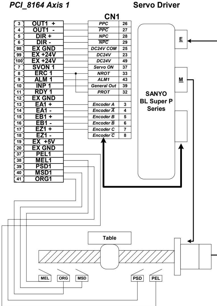
**Figure 7-3: Connection of PCI-8164 with SANYO Driver**
