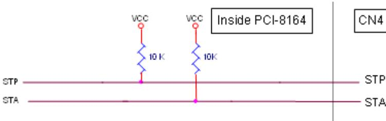
Both STP and STA signals are input and output signals. To operate the start and stop action simultaneously, both software control and external control are needed. With software control, the signals can be generated from any one of the PCL6045. You can also use an external open collector or switch to drive the STA/STP signals for simultaneous start/stop.
