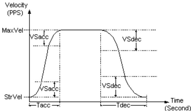
Normally, the accel/decel period consists of three regions: two VSacc/VSdec curves and one linear. During VSacc/VSdec, the jerk (second derivative of velocity) is constant, and during the linear region, the acceleration (first derivative of velocity) is constant. In the first constant jerk region during acceleration, the velocity
