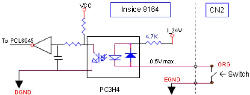
When the motion controller is operated in the home return mode, the ORG signal is used to inhibit the control output signals (OUT and DIR). For detailed operations of the ORG signal, refer to section 4.3.3.
