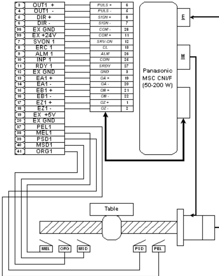
**Figure 7-2: Connection of PCI-8164 with Panasonic Driver**
