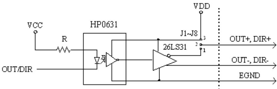
**NOTE** When the pulse output is set to open collector output mode, OUT- and DIR- transmits OUT signals. The sink current must not exceed 20 mA on the OUT- and DIR- pins. By default, pin 1-2 of the jumper is shorted.
