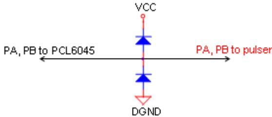
If the signal voltage of the pulser is not +5V or if the pulser is distantly placed, it is recommended that a photocoupler or a line driver be installed in between. Note that the CN3 +5V and DGND lines are provided from the PCI bus, and that this source is not isolated.
