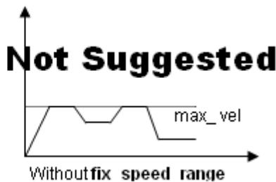
2. During the acceleration or deceleration period, using `_8164_v_change()` is not recommended. Even if it does work in most cases, the acceleration and deceleration time is not guaranteed.
