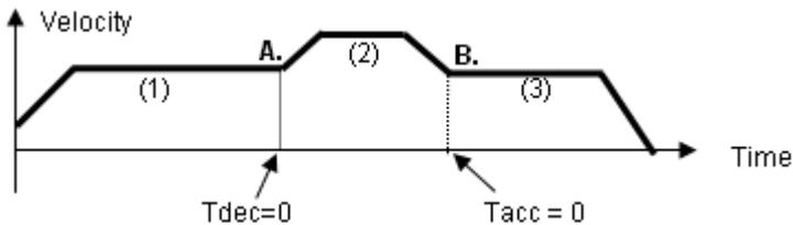
This example demonstrates how to use the continuous motion function to achieve velocity changing at pre-set points. The 1st motion ( $t_a$ ) moves the axis to point A, with  $T_{dec}=0$ , and then the 2nd continues immediately. The start velocity of (2) is the same with max velocity of (1), so that the velocity continuity exists at A. At point B, the  $T_{acc}$  of (3) is set to be 0, so the velocity continuity is also continued.
