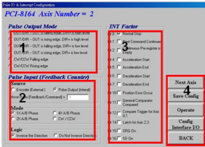
1. **Pulse Output Mode:** Selects the output mode of the pulse signal (OUT/ DIR). The related function call is `_8164_set_pls_outmode()`.
