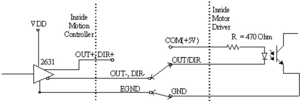
**WARNING** The sink current must not exceed 20 mA to prevent damage to the PCI-/MPC-/PXI-8164 card!
