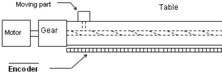
If this ratio is not set before issuing the start moving command, it will cause problems when running in “Absolute Mode” because the 8164 won’t recognize the actual absolute position during motion.
