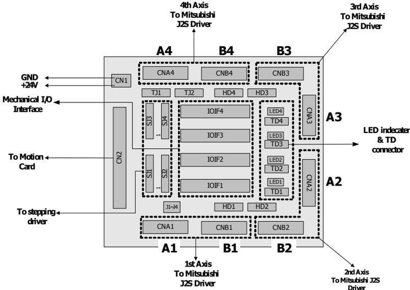
2. **CAN or CNB cables:** Two 20-pin cables (pin-to-pin) are required to connect the CNA and CNB with the Mitsubishi J2S driver. The required cables are available from ADLINK.
