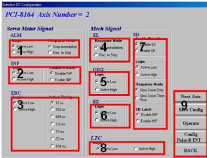
1. **ALM Logic and Response mode:** Selects the logic and response modes of ALM signal. The related function call is `_8164_set_alm()`.
