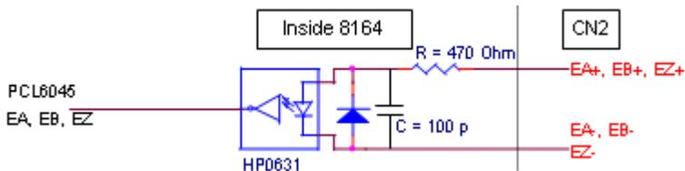
Note that the voltage across each differential pair of encoder input signals (EA+, EA-), (EB+, EB-), and (EZ+, EZ-) should be at least 3.5V. Therefore, the output current must be observed when connecting to the encoder feedback or motor driver feedback to avoid
