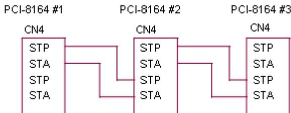
The following diagram shows how to allow an external signal to initiate the simultaneous start/stop connect a 7406 (open collector) or an equivalent circuit.
