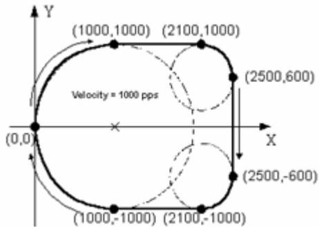
This example demonstrates how to use continuous motion function to achieve 2-axis continuous interpolation. In this application, the velocity continuity is the key. Refer to the previous example.
