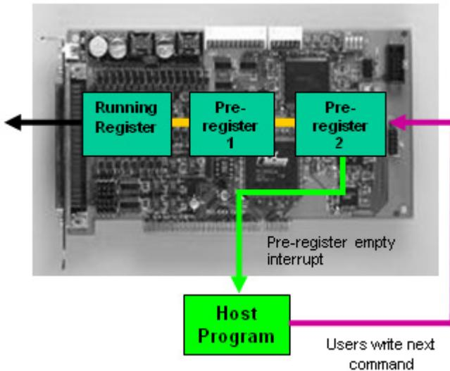
1. The first motion is executed and the CPU writes corresponding values into Pre-Register2.
