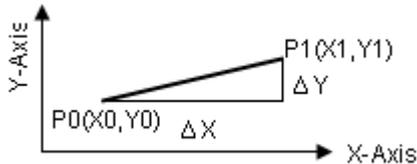
The speed ratio along X-axis and Y-axis is ( $\Delta X$ :  $\Delta Y$ ), respectively, and the vector speed is:
