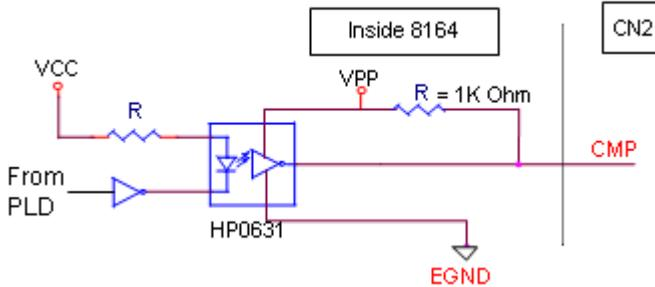
**NOTE** CMP trigger type may be set to normal low (rising edge) or normal high (falling edge). Default setting is normal high. Refer to function `_8164_set_trigger_type()` in section 6.16 for details.
