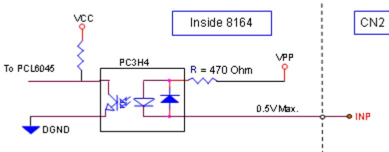
The in-position signal is usually generated by the servomotor driver and is ordinarily an open collector output signal. An external circuit must provide at least 5 mA current sink capabilities to drive the INP signal. For more details of INP signal operations, refer to section 4.2.1.
