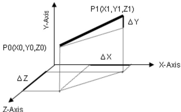
The speed ratio along X-axis, Y-axis, and Z-axis is ( $\Delta X$ :  $\Delta Y$ :  $\Delta Z$ ), respectively, and the vector speed is:
