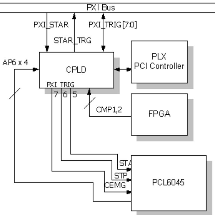
If you want to connect STA, STP, and CEMG to the PXI trigger bus, they can only set it to channel 5, 6, and 7, individually. STA may also be connected to PXI\_START by function selection. Also, PXI\_START's status could be read back through this function.
