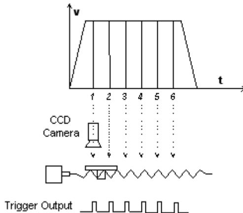
In this application, the table is controlled by the motion command, and the CCD camera is controlled by the position comparison output of the 8164. An image of the moving object is easily obtained.
